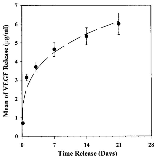
**FIGURE 1.** Cumulative release of VEGF from the PLGA delivery device in 0.5 ml of 0.9% sodium chloride saline at 37°C. These data are fitted to a power function of time  $t$ ,  $f(t) = kt^n$ , using a nonlinear square fit algorithm<sup>32</sup>;  $k = 2.57 \pm 0.031$  and  $n = 0.29 \pm 0.05$ . This suggests that the VEGF release was governed by diffusion-like process.
