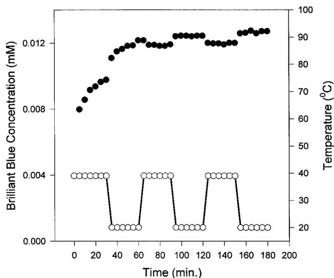
**Figure 5.** The composite membrane loaded with brilliant blue was transferred to a thermal bath. The concentration of brilliant blue in the bath was monitored by determining turbidity of the bath by using a spectrophotometer. Drug release increased exponentially to a final value that is temperature dependent.
