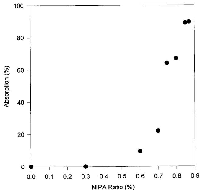
**Figure 1.** The water absorption of the silicone rubber/N-isopropylacrylamide (SR/NIPA) composite material was measured as a function of the ratio of NIPA particles incorporated over the composite material in volume. The threshold of absorption was identified at a ratio of approximately 75%.
