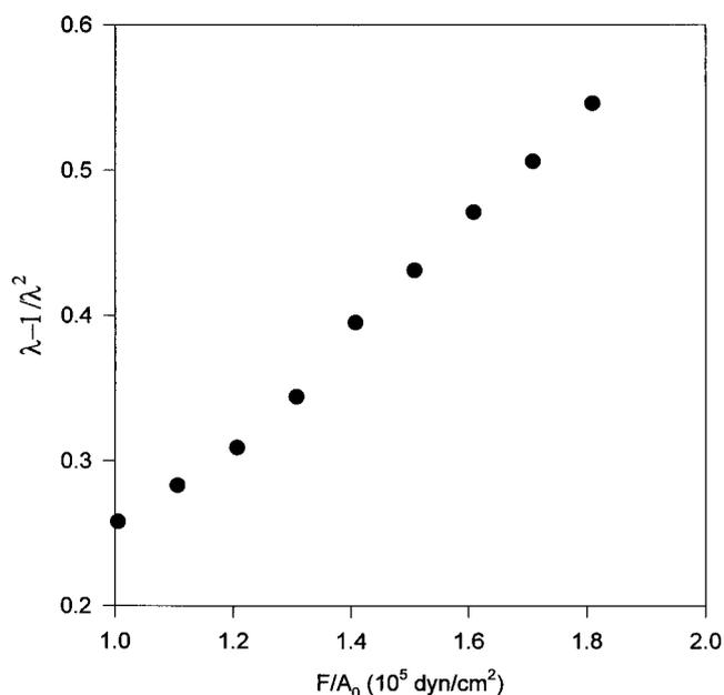
**Figure 3.** The shear modulus of the composite material was measured by the tensile method and found to be  $3.6 \times 10^5$  dyn/cm<sup>2</sup> for the sample containing 85% NIPA.
