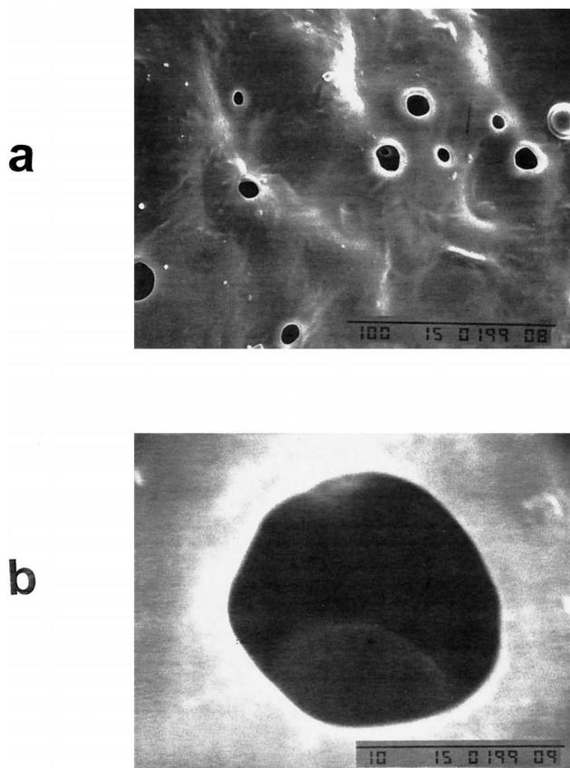
**Figure 4.** The surface of the composite membrane was studied by scanning electron microscopy. Samples were first dried and then coated with gold. (a) Attached inside the voids of silicone rubber are NIPA gel particles in the dehydrated state. (b) Close-up of a single NIPA particle embedded in the surface of the silicone rubber membrane.
