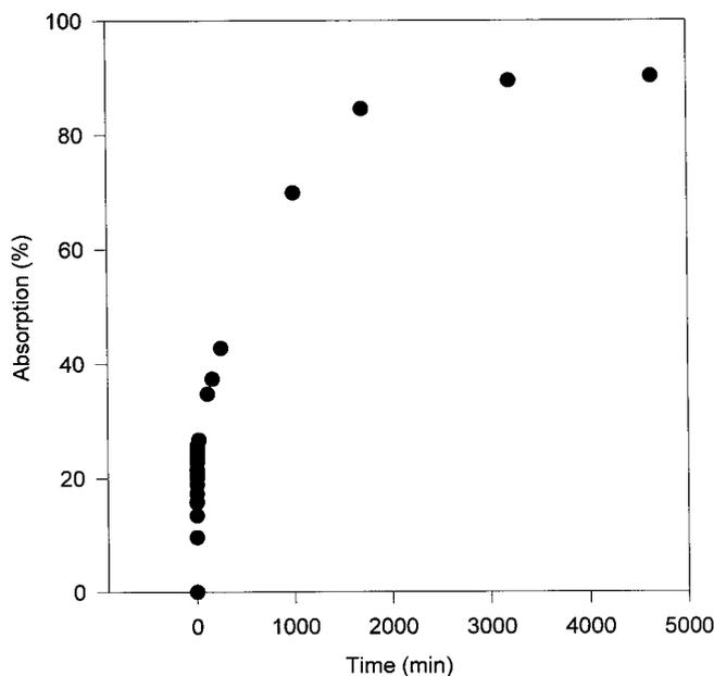
**Figure 2.** Water absorption of the composite membrane at an 85% ratio, with a thickness of 0.65 mm, was measured as a function of time. The absolute absorption time depends upon the ratio of NIPA to SR and the thickness of the composite membrane.
