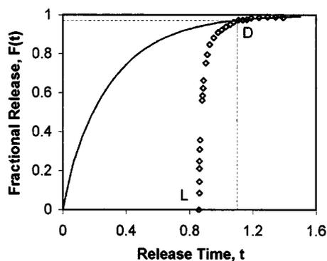
FIGURE 3. Fractional-release profiles. The squares are existing data of [Ref. 11, Fig. 6(c), millirods 1]. The trypan blue is released from PLGA rods into a PBS medium. The solid line is calculated by Eqs. (14)–(16), with  $t_L=0.859$ ,  $D=1.91 \times 10^{-9} \text{ cm}^2/\text{s}$ ,  $S=3$ , and  $k=1$ .
