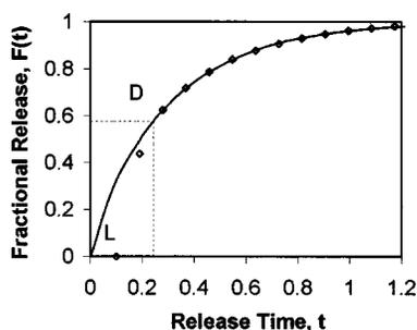
**FIGURE 1.** Fractional-release profiles. The diamonds are the Nadia 3.3–50 data set, described in the experimental section. The BSA is released from PLLA (200 kD) fibers, into a phosphate buffered saline. The solid line is calculated by Eqs. (14)–(16), with  $t_L=0.101$ ,  $D=9.244 \times 10^{-13}$  cm<sup>2</sup>/s,  $S=3$ , and  $k=1$ .
