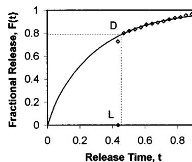
FIGURE 5. Fractional-release profiles. The diamonds are the MWCAl Veena 200/20 data set, described in the experimental section. The BSA is released from PLLA (200 kD) fibers, into a phosphate buffered saline. The solid line is calculated by Eqs. (14)–(16), with  $t_L=0.435$ ,  $D=4.532 \times 10^{-13} \text{ cm}^2/\text{s}$ ,  $S=3$ , and  $k=1$ .
