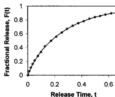
**FIGURE 2.** Fractional-release profiles. The diamonds are existing data of [Ref. 16, Fig. 1, empty circles]. The leavamisole is released from poly( $\epsilon$ -caprolactone) (147 kD) rods into a medium similar to that encountered in the rumen of cattle medium. The solid line is calculated by Eqs. (14)–(16), with  $t_L = 0.00315$ ,  $D = 1.222 \times 10^{-7}$   $\text{cm}^2/\text{s}$ ,  $S = 3$ , and  $k = 1$ .
