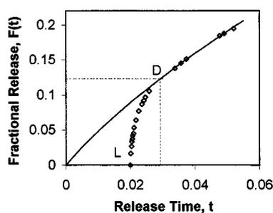
FIGURE 4. Fractional-release profiles. The diamonds are existing data of [Ref. 10, Fig. 2(B), TES]. The testosterone is released from PLLA rods into a dichloromethane medium. The solid line is calculated by Eqs. (14)–(16), with  $t_L=0.02$ ,  $D=4.04 \times 10^{-10} \text{ cm}^2/\text{s}$ ,  $S=3$ , and  $k=1$ .
