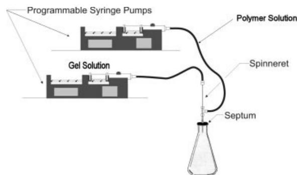
**FIGURE 1** Diagram of the extrusion apparatus used to create the fibers discussed in this article. Polymer and solutions contained in syringes were concurrently extruded using two linear syringe pumps. Appropriate fittings and tubes connected each syringe to a dual-lumen spinneret designed for these extrusions.
