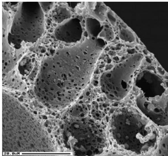
**FIGURE 2** SEM taken at 1000 $\times$  magnification, 15.0 kV, detailing the wall cross-section of a hydrogel-cored, PLLA blend fiber incorporating a 10% aqueous phase incorporated as an emulsion within the polymer shell. Bar represents 20  $\mu\text{m}$ .
