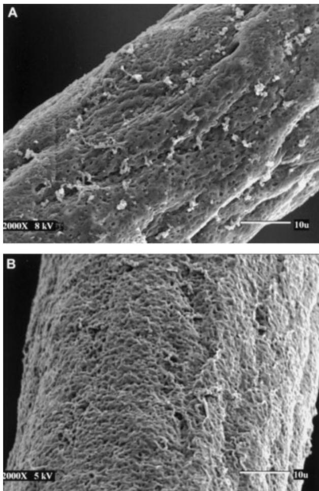
**Figure 2.** Scanning electron microscopy depicting surface morphology for PLLA fibers (A) and ECM gel-coated PLLA fibers (B), at an original magnification of 2000 $\times$ . Scale bar represents 10 microns.
